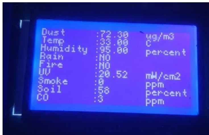
Figure 9: LCD screen displaying measured environmental parameters
